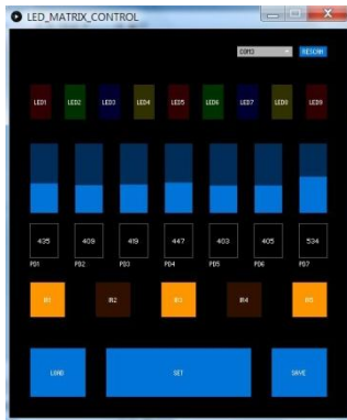
Figure 4. The output MSP signals shown by control software
