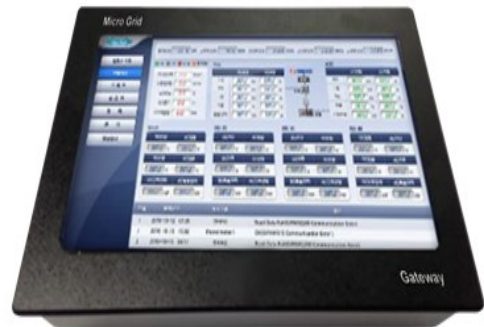
Figure 3 Gateway for Microgrid
